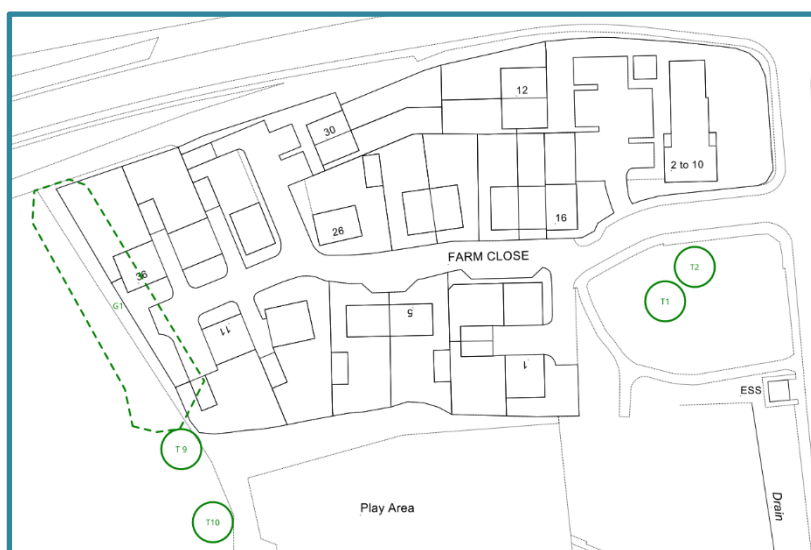
Figure 2. Plan showing trees that are protected by TPO's and successfully retained and incorporated into a newly completed development
